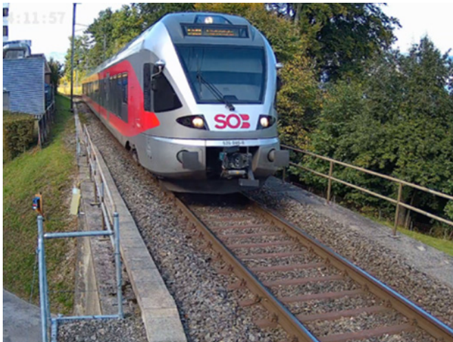
Figure 2: Camera recording of a train to capture train type, speed and composition.
