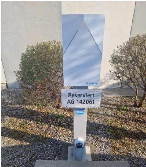
Abbildung 5: WiTricity Halo Wireless Charger 11 kW Wall Box
