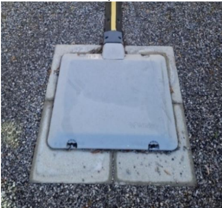
Abbildung 4: WiTricity Halo Wireless Charger 11 kW Ground Pad
