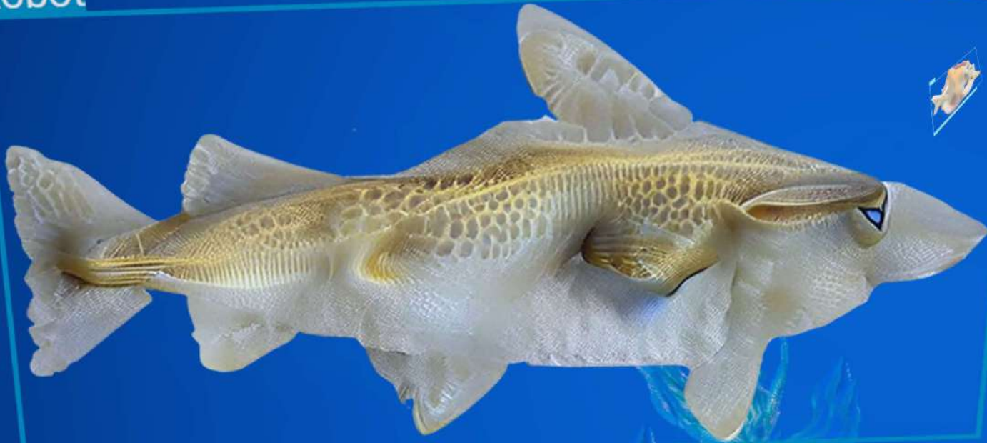
3DPU2 - 3D-printed underwater robot in the shape of a codfish
